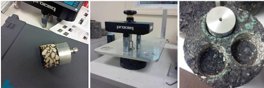
150 mm diameter test cylinder with three 50 mm diameter cut-outs.
