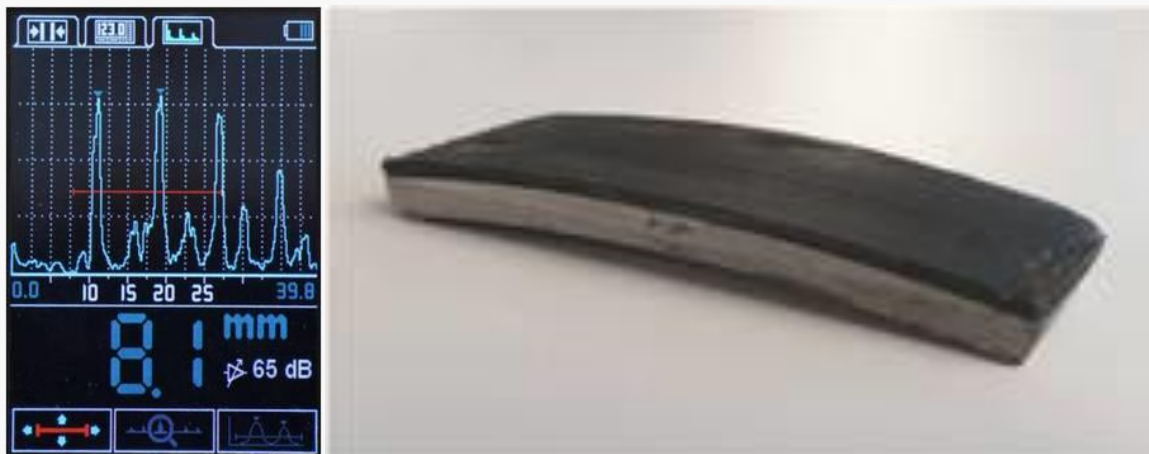
Display shows output of the measuring, shown as 8.1 mm. Any erosion or corrosion on the steel inner surface would show a lower value.
