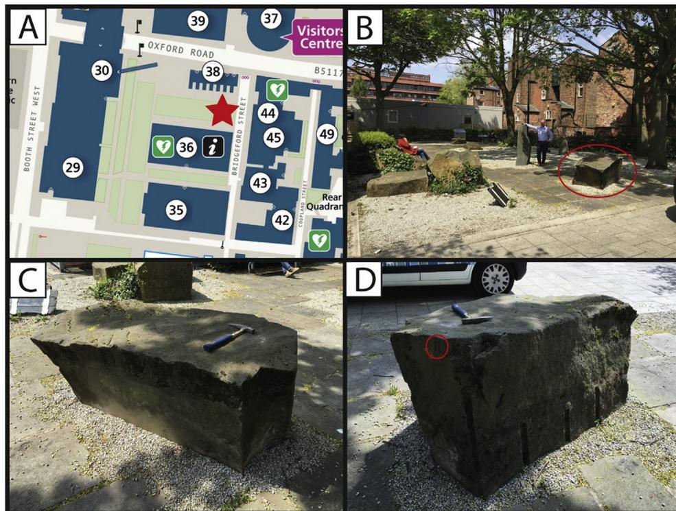
**Fig. 1.** A) Red star denotes the location of the rock garden. B) Location of the SHED calibration boulder. C & D) Views of the sandstone calibration boulder. Red circle shows etched #11. Rock hammer for scale. (For interpretation of the references to colour in this figure legend, the reader is referred to the web version of this article.)
