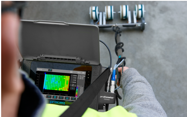
Profometer Corrosion with a 4 wheel electrode
