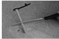
Cut sleeve according to measuring depth
