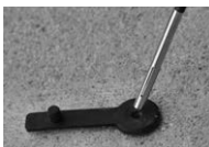
Insert In-Situ probe into sleeve
