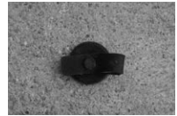
Insert sleeve in test hole and close cap
