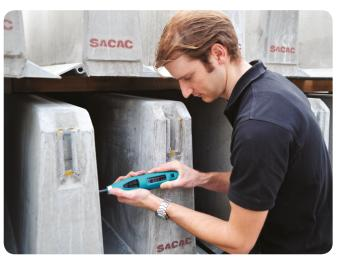
**ST/PC Type N/L:** The world's most advance rebound hammer, with unmatched dispersion characteristics, durability and measuring range.
