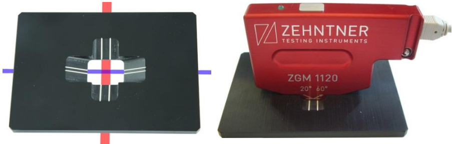
Positioning support example for measurements on small parts
